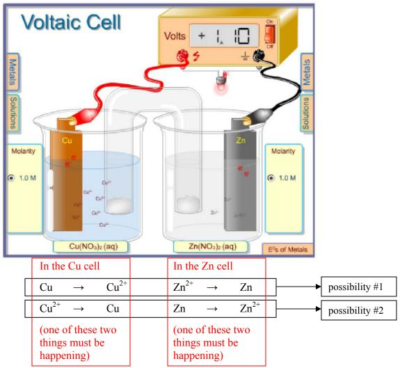
...use the reduction potentials to figure out which one of these cells is the oxidation (anode) and which is the reduction (cathode)
